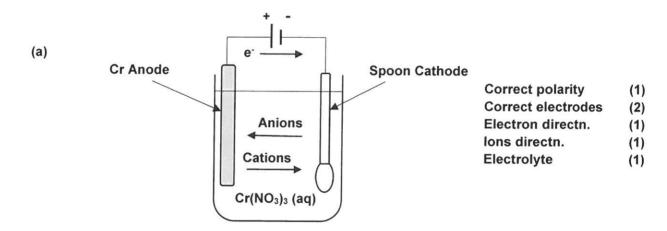
(b) At the cathode, the negative terminal of the cell provides electron for the reduction of chromium ions to chromium metal being deposited on the spoon. (1)
